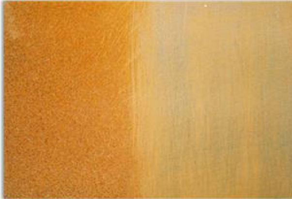
Hand Tool Cleaned to SSPC-SP2 Standard
