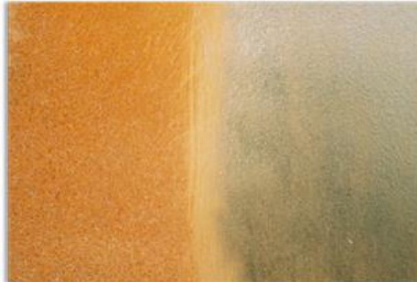
Power Tool Cleaned to SSPC-SP3 Standard
