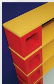
Step eight Place each shelf across two blocks, fixing with a generous blob of construction glue. Stack alternate blocks and shelves, as shown. Leave glue to dry before using.
