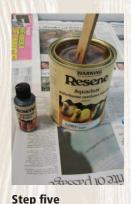
Carefully pour the Resene Colorwood Enhance into the Resene Aquaclear and stir well with a paint
