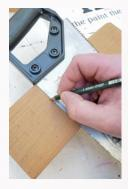
Step one Mark the piece of timber into five equal cubes.
