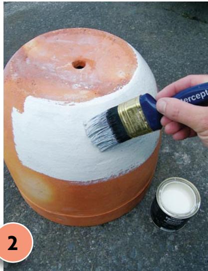
2 Apply one coat of Resene Terracotta Sealer to the inside and outside of the pot. Allow to dry for at least six hours.
