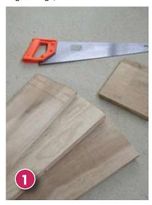
Use the saw to cut the plywood to the dimensions listed above.
