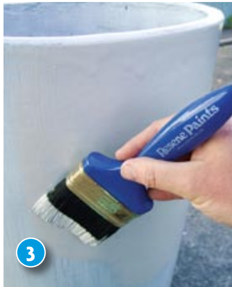
3 Apply one coat of Resene Silver Chalice (Lumbersider) to outside, rim and inner rim of the pot. Allow to dry for about two hours.
