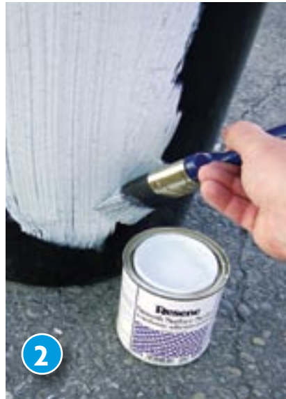
2 Apply one coat of Resene Smooth Surface Sealer to the glazed surface of the pot, ensuring an even coverage. Allow to dry for about two hours
