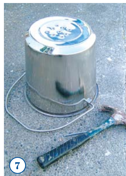
7 USING the hammer and large nail, punch a series of drainage holes in the bottom of the stainless steel bucket.
