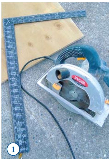
1 USING a skilsaw or handsaw, cut a panel of ply measuring 550mm x 850mm.
