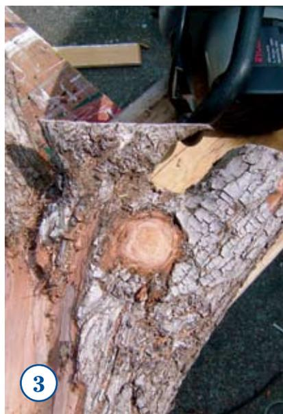
**3** WITH a chainsaw, carefully remove any unwanted knots, lumps or small branch stumps.
