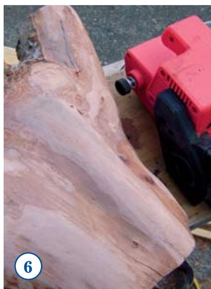
**6** LIGHTLY sand using the belt sander, first with a coarse grade sanding belt, then with a medium grade.
