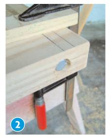
TAKE one of the non-drilled lengths of timber and apply PVA to one end. Place this against one of the drilled lengths of timber and clamp together to form a right angle. Use the long 8mm drill bit to drill through the 10mm hole and into the second piece of timber. Use the ratchet to screw in the 150mm coach screw, as shown. Repeat with the other three corners to form the outer frame.
