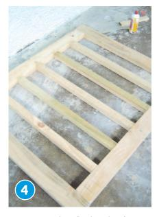
MEASURE and cut five lengths of 50mm x 50mm timber and evenly space them, as shown. Fix to the outer frame using PVA glue.
