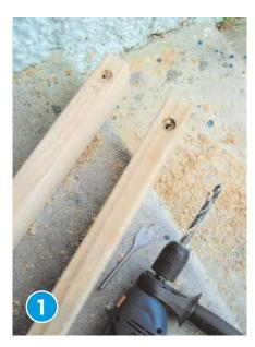
TAKE two of the 1m lengths of timber and, using the 25mm flat wood bit, drill four holes approx 50mm from each end – this is to countersink the coach bolts, so only drill to about 10mm deep. Drill a hole through the centre of each of these using the 10mm drill bit.
