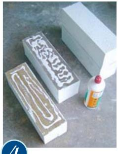
GLUE the bare wood faces of the base plinths together using exterior wood glue. Allow to dry completely.
