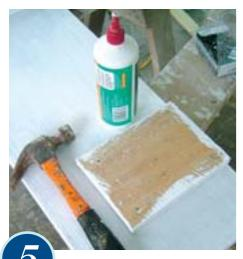
ATTACH the dividers to each seating plank with glue and 50mm galvanised nails, positioning them 100mm in from each end.
