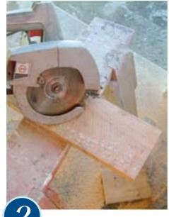
CUT eight 200mm lengths from the fence paling to form the seat dividers. Cut four 320mm lengths from the fence post to form the base plinths.
