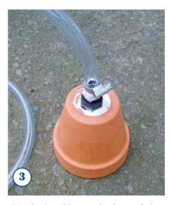
FIX plastic tubing to the base of the small terracotta pot using the plastic male coupling, silicon sealant and galvanised hose clip. Allow sealant to cure overnight.
