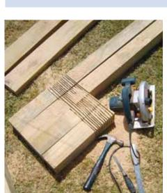
SET the skill saw blade to a depth of 50mm and cut two lines across the four legs 350mm and 450mm from bottom. Cut a series of close lines across the four legs and remove with a hammer and chisel.
