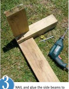
the front legs, then drill a 100mm hole as shown and bolt the front beam to the front legs. Repeat with the back legs and back beam.
