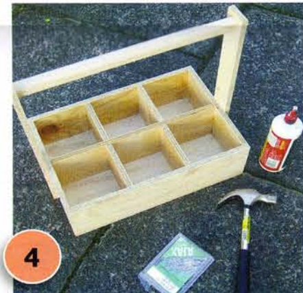
4 Position the handle supports, fixing with PVA and panel pins. Position the cut dowel between them, as shown, securing with PVA glue and panel pins. Punch in nail heads with a nail punch and fill holes with filler. Once dry, sand smooth.
