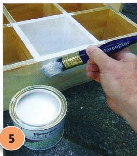
5 Apply one coat of Resene Quick Dry to the entire carry tray and allow to dry for one hour.
