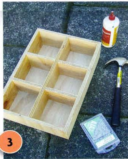
3 Fix the base into position using PVA and panel pins, nailing through from underneath.
