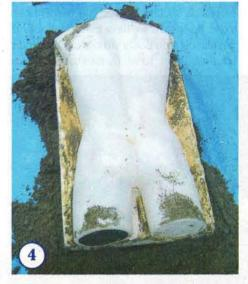
ONCE the plaster is dry, remove the frame and clay, turn the mannequin and mould over and repeat the process to cast the mould for the back.
