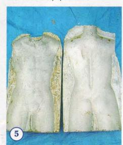
CAREFULLY remove each half of the plaster mould from the mannequin and fill any air bubbles or imperfections with plaster.
