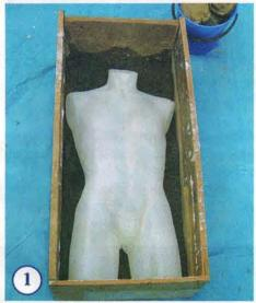
CONSTRUCT a box frame large enough to contain the torso and place it face up on a layer of sand. Pack sand around the torso to a level halfway up each side.
