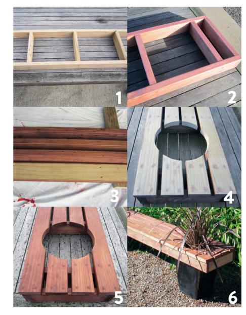
Mark the position of the ends and the internal struts on the frame front and back. The gap between the end and the first internal strut should be about 70mm, followed by a gap large enough to fit your pot, repeat at the other end and centre the remaining struts.
