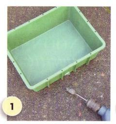
Drill a 25mm hole in the side of one of the plastic boxes, near the base, as shown.
