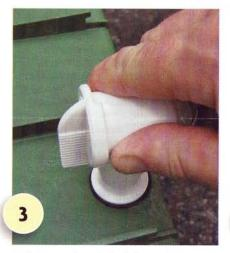
Push the tap through the hole, as shown, and fix from behind with the brass nut back.
