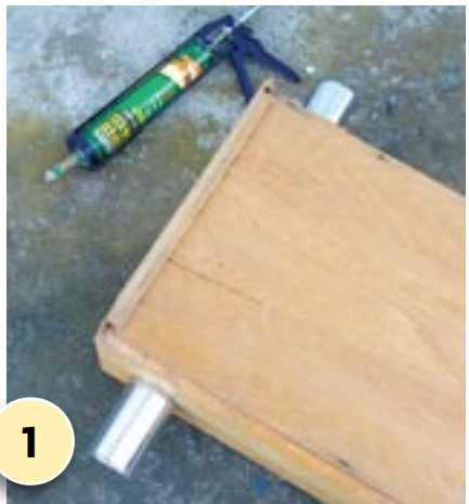
1 Remove all can labels and sand the cans lightly. Then, to make arm 'sockets', attach two small tins to the wooden drawer sides, as shown, using the glue and a small screw through the base (make a pilot hole first with the drill or nail punch).
