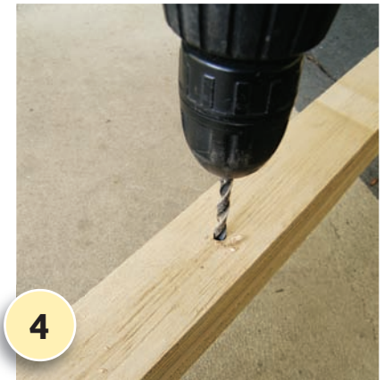
4 Clamp the two longer legs together. Drill a 5mm hole through both, about 260mm from one end and drill two 5mm holes in the sides of the tray about 65mm from one end. Unclamp. Bolt each leg to the tray.
