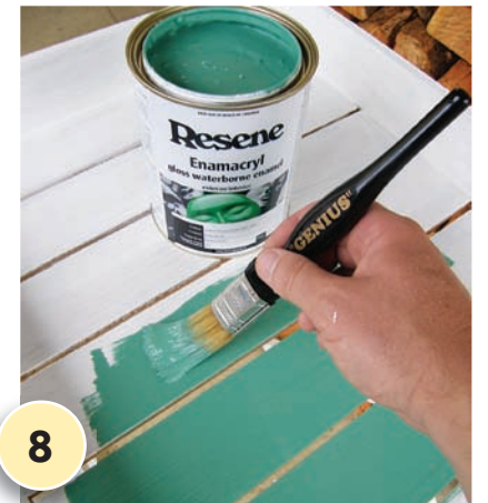
8 Apply two coats of Resene Green Room to the tray, allowing two hours for each coat to dry. Drill 10mm holes approximately 35mm from the end of each front leg and attach wheels with 60mm bolts/washers and nylock nuts.
