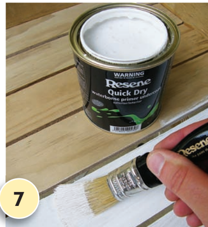
7 Glue and screw the second pair of legs to the tray and then attach their support bar – in the same way as the other legs' support bar. Once glue has dried, apply a coat of Quick Dry to the entire tray, allowing two hours to dry.
