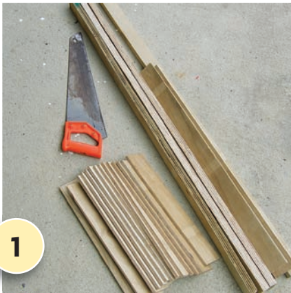
1 Measure and cut plywood and dowel to the dimensions listed above. Smooth rough edges with sandpaper.
