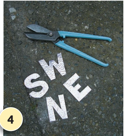
4 Cut the letters N, S, E, and W out of the stucco aluminium, as shown, using the marker to outline the letters first. Wipe them clean afterwards with a cloth. Then cut out a 'head' and 'tail' for the pointer and a kiwi shape.
