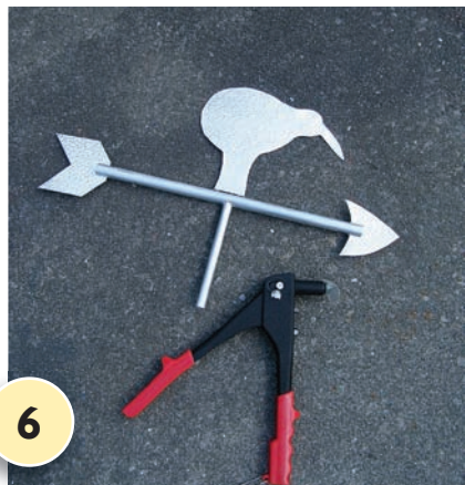
6 Slide the pointer's head and tail into the slit at each end of the pointer's horizontal bar. Fix with construction glue. Attach the letters to the main frame the same way. Fix the kiwi to the horizontal bar with pop rivets (follow the manufacturer's instructions).
