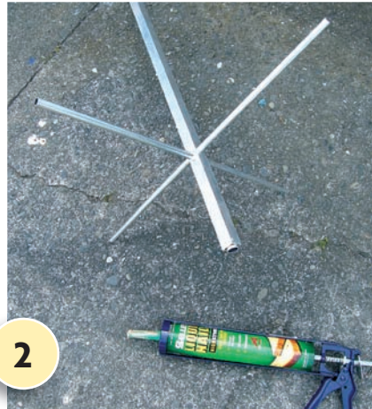
2 Slide the second piece of tubing into place, as shown. Cut a 150mm length of the 16mm tubing. Slide this inside the top of the square aluminium. Fix it with a small amount of construction glue, taking care not to get glue on the inside of the 16mm tubing.
