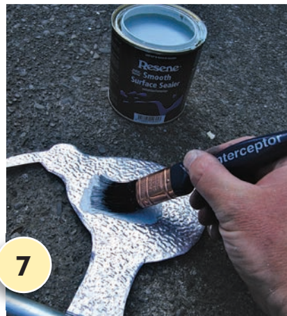
7 Allow glue to dry and then apply one coat of Resene Smooth Surface sealer to the weather vane, allowing two hours for it to dry. Don't apply sealer to the vertical bar of the pointer.
