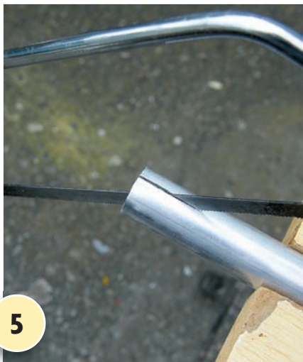
5 Use the hacksaw to cut a 15mm vertical slit in each end of the horizontal bar of the pointer, as shown.
