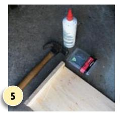
Fix the roof overhang to the roof with PVA and nails — always drill 1.5mm pilot holes before nailing to prevent the plywood from splitting.
