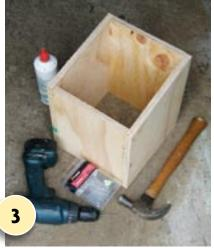
Assemble the four walls, as shown, fixing along the edges with PVA glue and galvanised nails. Sand or lightly file the rear wall's top edge so it aligns with the pitch
