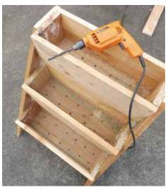
**STEP NINE**Drill drainage holes in the base of each planter box, as shown.
