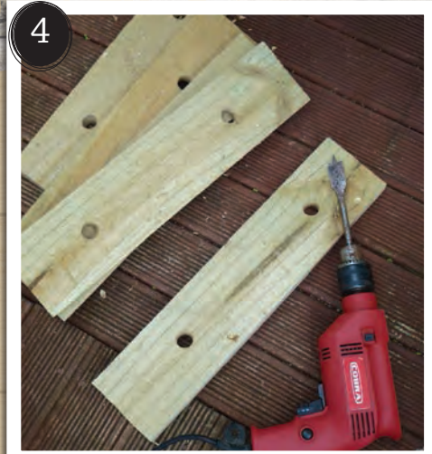
Drill two drainage holes in each base, as shown.
