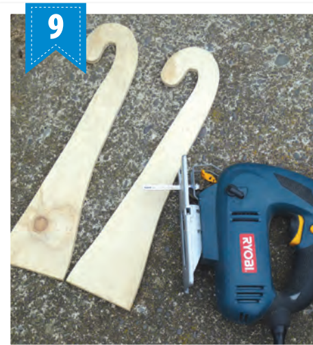
Cut out both handles with a jigsaw and smooth any rough edges with sandpaper.
