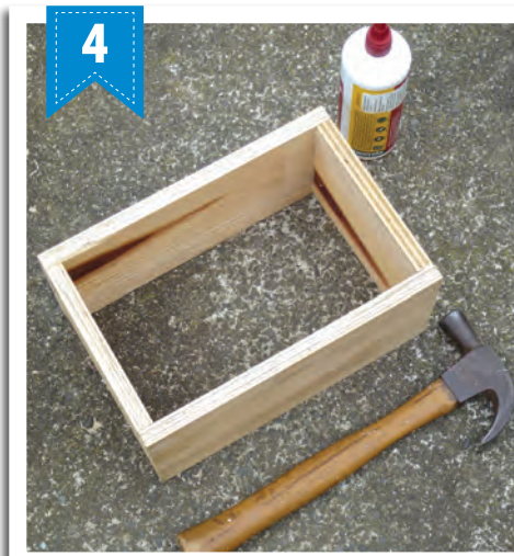
On a flat surface, assemble the sides of the box, as shown, fixing along each edge with PVA glue and 25mm nails.
