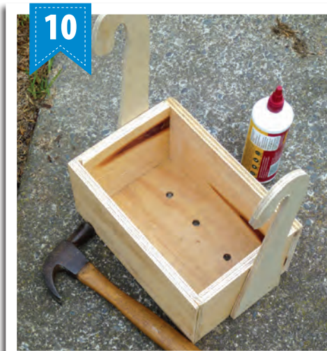
Drill six 10mm drainage holes in the base of the box and fix the two handles into position, as shown, attaching with PVA glue and 25mm nails.
