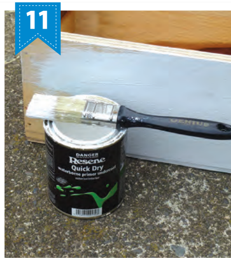
Apply one coat of Resene Quick Dry to the peg box and allow two hours to dry.
