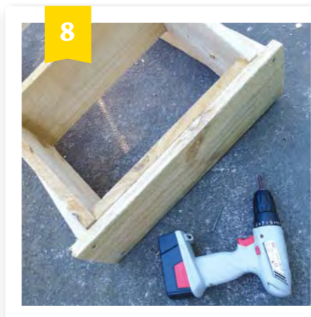
Measure, mark and cut a piece of fence paling approximately 540mm and attach to the top of the display ladder, as shown, overlapping each side evenly. Fix with PVA glue and 65mm screws.
