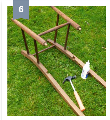
Continue reassembling the legs and back of the chair, fixing each joint with PVA glue. Gently tap with a hammer, if necessary, to ensure joints are firmly in position.
