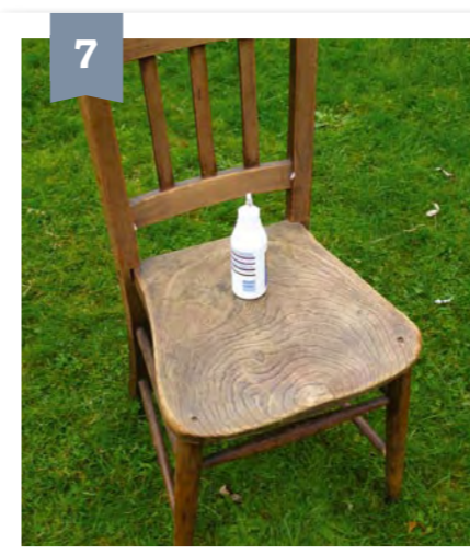
Place the seat in position, fixing with PVA glue.
