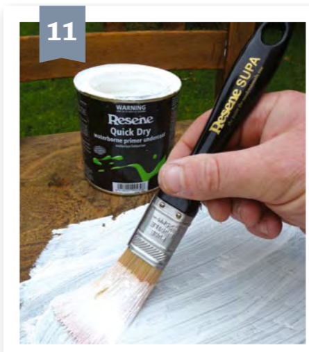
Apply one coat of Resene Quick Dry to the chair and allow two hours to dry.
