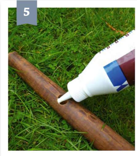
Apply a generous amount of exterior PVA glue to each of the chair joints and begin to reassemble.
