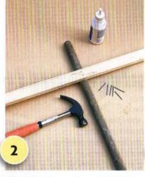
Attach the larger piece of battening across the broom handle, fitting it into the cut out section, as shown. Fix with two nails and PVA glue.
