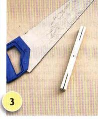
Cut two 60mm slots down either end of the other piece of battening, as shown, and drill a 4mm hole in the centre.
