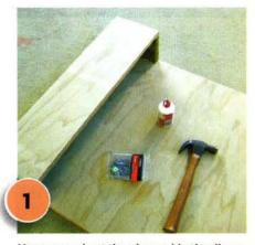
Measure and cut the plywood in the dimensions listed. Smooth rough edges with sandpaper. Assemble the window box's front, sides and base and fix with PVA glue and nails. Attach the box to the main backing board, as shown.
