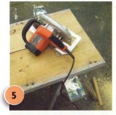
Cut two 180cm lengths and four 45cm lengths from the 300mm x 50mm timber. Smooth any rough edges with sandpaper.
