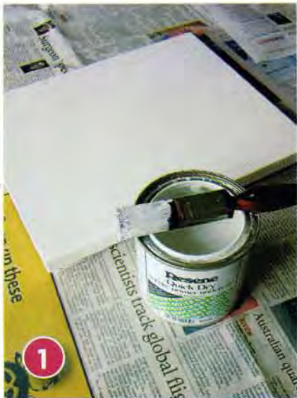
1 Apply one coat of Resene Quick Dry primer to the front, back and edges of the plywood board. Leave to dry for at least one hour.
