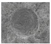
Cement and paint paste air bubble at 2500x magnification.
