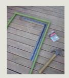
STEP SIX Attach two of the 600mm lengths to two of the 1200mm lengths to form a rectangle, fixing with 40mm nails and PVA glue. Use the set square to ensure the corners are at right angles.
