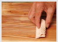
4. Using the graining rocker. Pull the graining rocker down slowly, and rock it backwards and forwards as you move it down to create knots in the wood. Make the knots at random intervals.
